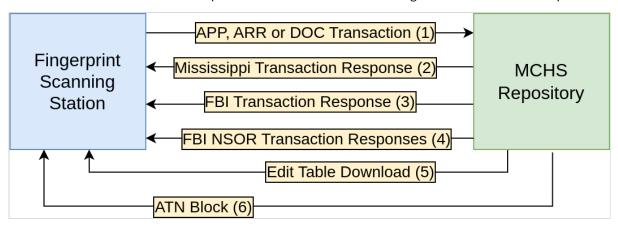
The diagram above shows the flow of information between a fingerprint scanning station (livescan or cardscan) and MCHS. The primary flow consists of a scanning station:
